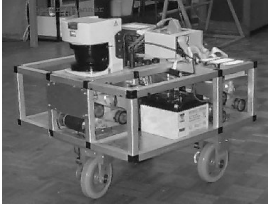
Figure 2: The test vehicle. The laser range finder is seen in the front
